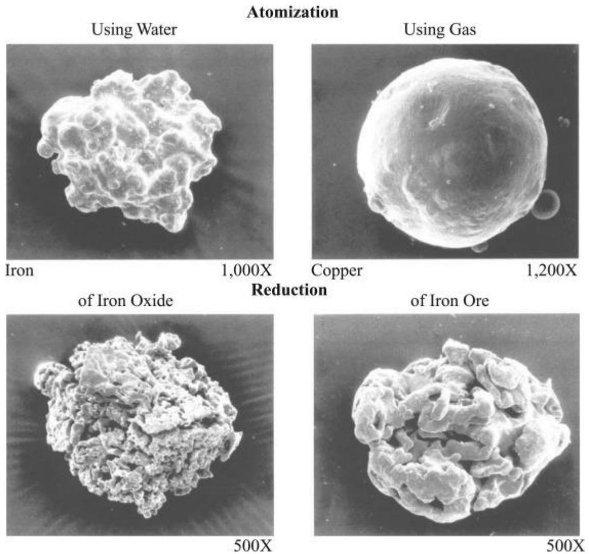
Figure 1. Morphology of metal powders made by various manufacturing processes (atomization/reduction).
